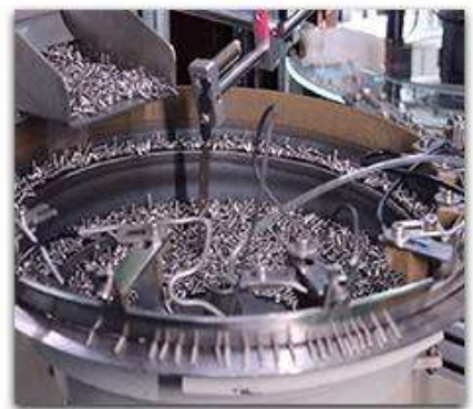
电脑选钉机 Computer nail selection machine
